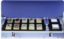
Quick Ray Master is an automated tissue microarrayer running by the built-in PC.
