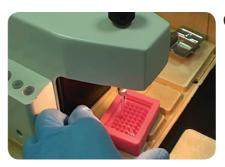
02 Dispense liquid paraffin (60~65°C) slowly into the mold kit until the top of core rods are fully submerged.
