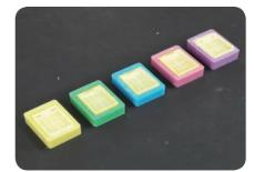
**05** Solidify the embedding cassette and the mold kit at a normal room temperature or at about 4°C for 30~60 minutes.
